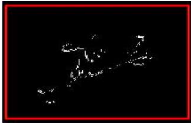
Fig. 1.2: Binary Image interpreting the bit value of 0 as black and 1 as White Features Extraction is the key to develop an offline signature recognition system. We use a set of five global features that cannot be affected by the temporal shift.
